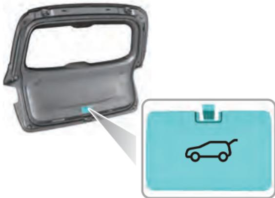
An emergency tailgate opening mechanism is located on the catch and can be accessed via a bespoke access point.
