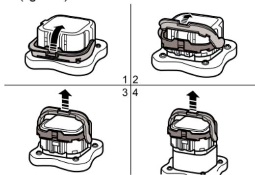
**Note:** After the manual service disconnect has been removed, please cover the open connector to prevent ingress of any debris or contaminants.
