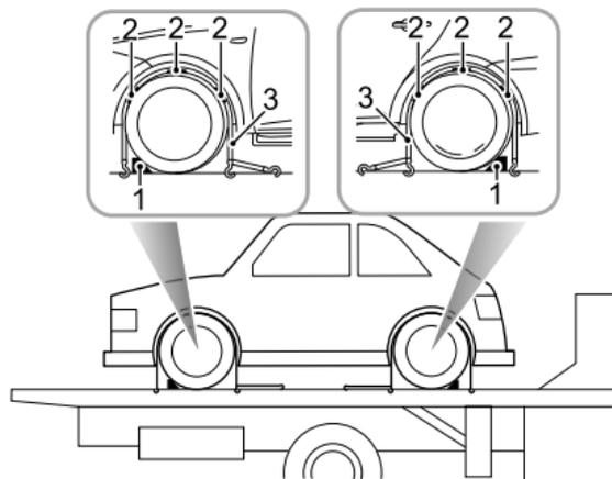
In cases where the vehicle breaks down or encounters an accident, you can use the towing hook to tow your vehicle, such as towing your vehicle onto the transporter. But they are not designed for towing other vehicles. The vehicle can be towed by using a soft rope, but a hard rod is recommended. Please consult the Owner's Handbook for detailed instructions.
